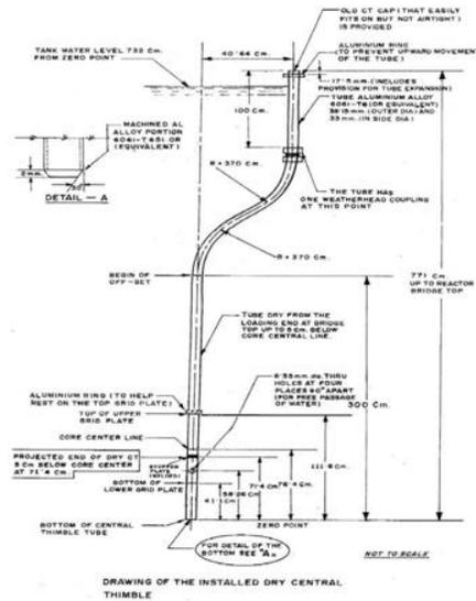
**Figure 2 : Schematic drawing of Dry CT tube for I-131 production**
