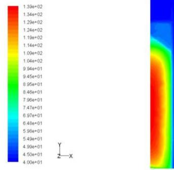
Figure 10.: Contours of static temperature ( $^{\circ}\text{C}$ )- Case-2 : Wet CT with holes over the Al-can and the RNG  $k-\epsilon$  model (Water Height : 2m)
