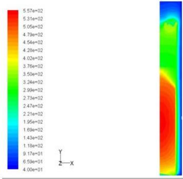
Figure 9.: Contours of static temperature ( $^{\circ}\text{C}$ )- Case-1: Dry CT tube with holes over the Al-can and the RNG  $k-\epsilon$  model
