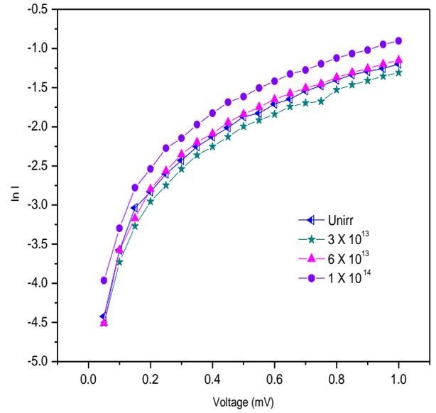
**Figure 6:** Semi logarithmic I-V characteristics of the as-deposited and irradiated Zr/n-Si samples
