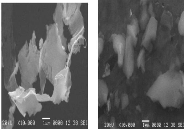
**Figure 2:** SEM micrographs of Zr–Si silicide films formed by ion irradiation at fluence: (a) no ions (b)  $3 \times 10^{13}$  ions/cm<sup>2</sup>, (c)  $6 \times 10^{13}$  ions/cm<sup>2</sup> and (d)  $1 \times 10^{14}$  ions/cm<sup>2</sup>.
