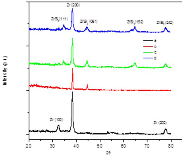
**Figure 1:** XRD spectra of the Zr–Si silicide films as a function of the irradiation doses, (a) virgin, (b)  $3 \times 10^{14}$ , (c)  $6 \times 10^{14}$  and (d)  $1 \times 10^{14}$  ions/cm<sup>2</sup>.
