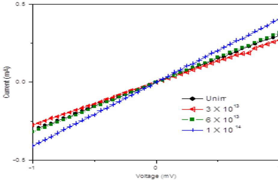
**Figure 5:** I-V characteristics of the as-deposited and irradiated Zr/n-Si samples showing the formation of Ohmic contact.
