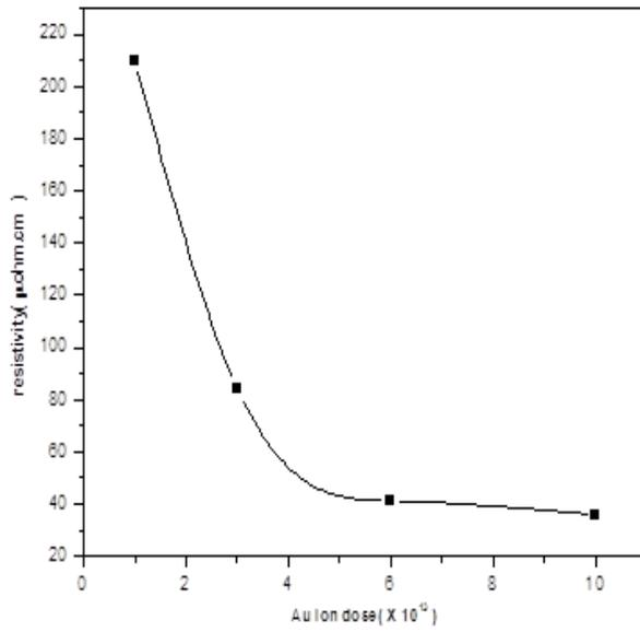
**Figure 4:** The variation of the resistivity of the Zr-Si silicide films as a function of the irradiation ion dose.
