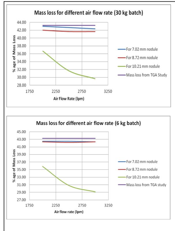
**Fig. 6: Mass loss with respect to different air flow rates.**
