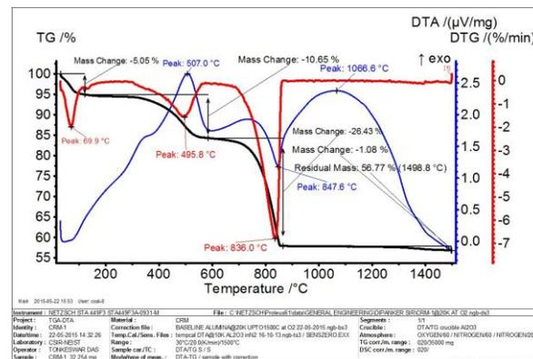
**Fig. 5: Total Mass loss observed in the TGA/DTG plot.**
