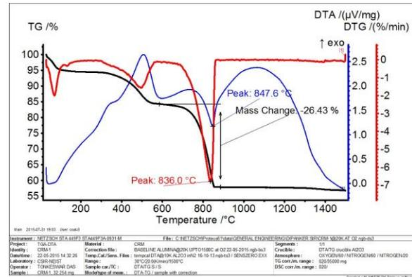
**Fig. 4: TGA/DTG plot of mass loss from calcination of limestone.**
