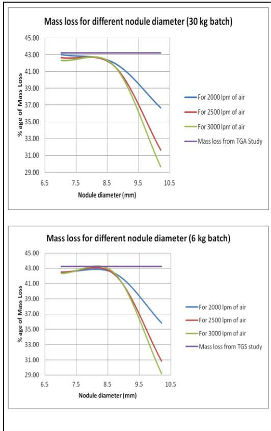
**Fig. 7: Mass loss with respect to different nodule diameters.**
