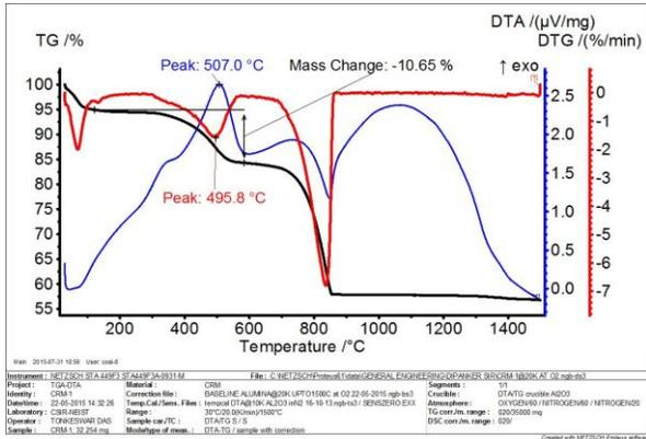
**Fig. 3: TGA/DTG plot of mass loss from combustion of coke breeze.**
