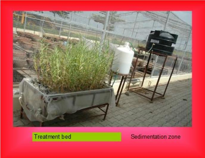
Fig. 1: Sub-surface horizontal wetland system including sedimentation and treatment zone.
