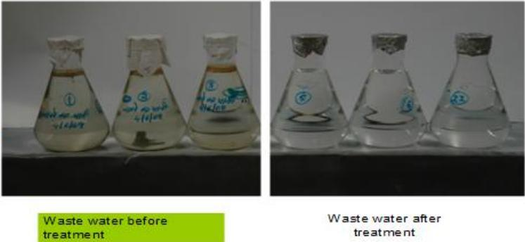
Fig. 3: Change in color of water before and after treatment of waste water.
