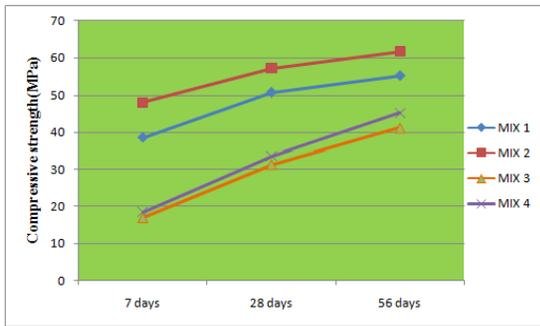
Fig. 1. Comparison of Compression strengths of all four mixes
