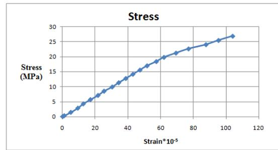
Fig. 5. Stress Strain curve for MIX 4
