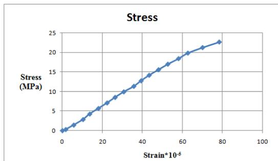
Fig. 4. Stress Strain curve for MIX 3
