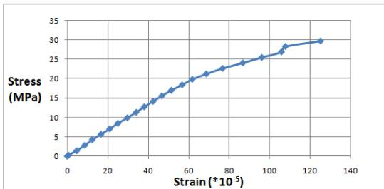
Fig. 3. Stress Strain curve for MIX2
