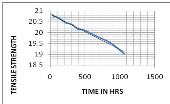
Fig 2: Graph for HDPE sample at different time span
