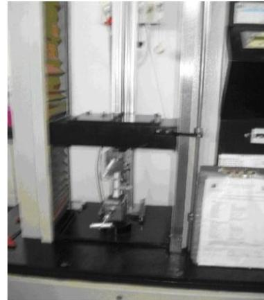
**Fig. 1: Universal Tensile tester.**
