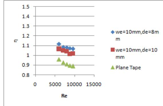
**Fig. 4: Variation of Enhancement for different inserts.**
