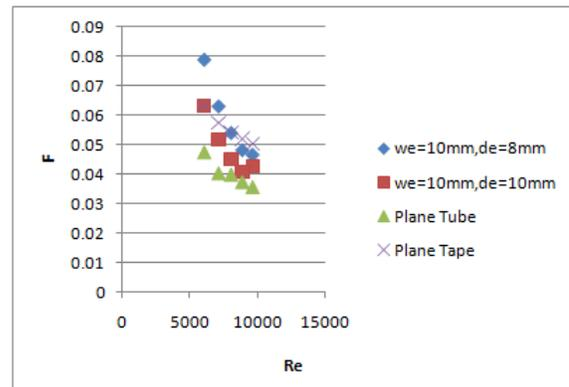
**Fig. 6: Variation of friction factor for various inserts:**
