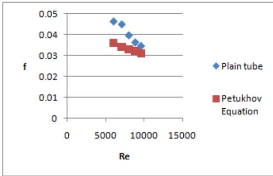
**Fig. 3: Validation results for Friction factor.**
