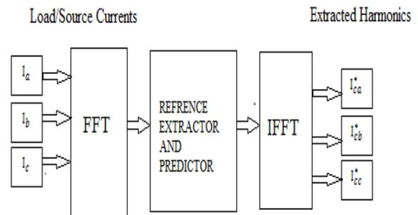
**Fig. 3.1: Block diagram of Fourier transform based extraction system.**
