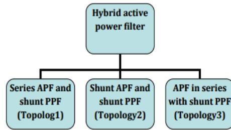
Fig. 1.1: General classification of hybrid active power filter.
