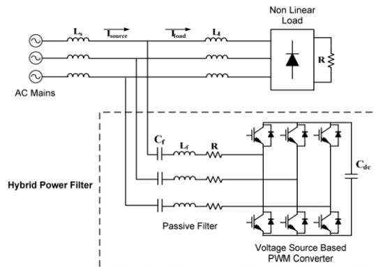
Fig. 2.1: Hybrid Active Power Filter.
