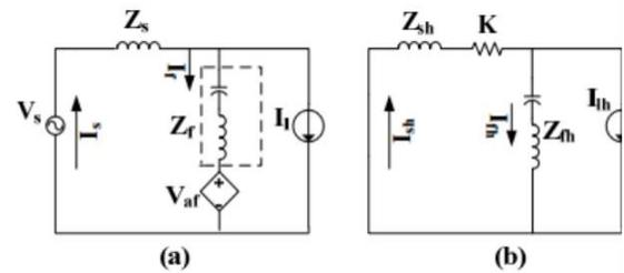
**Fig. 2.2: (a) Single Phase Equivalent Circuit (b) Harmonic Equivalent Circuit.**
