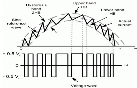
**Fig. 3.4: Principle of hysteresis bandwidth controller.**
