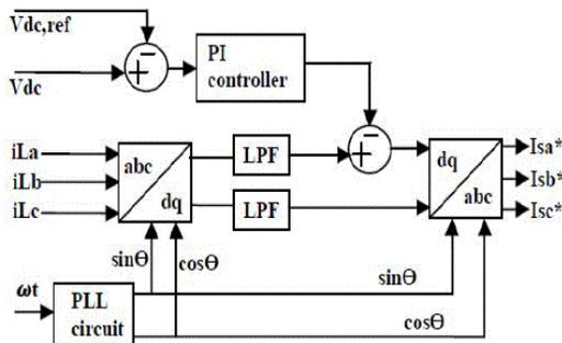
**Fig. 3.3: Synchronous reference frame method with direct control scheme.**
