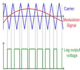
**Fig. 3.5: Principle of SPWM.**
