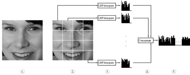
**Figure 1: Face description with local binary patterns.** 1. A registered face image is assumed. 2. The image is divided into local regions. 3. An LBP histogram is extracted independently from each region. 4. The histograms from regions are concatenated. 5. The concatenated histogram is used as descriptor for face recognition.
