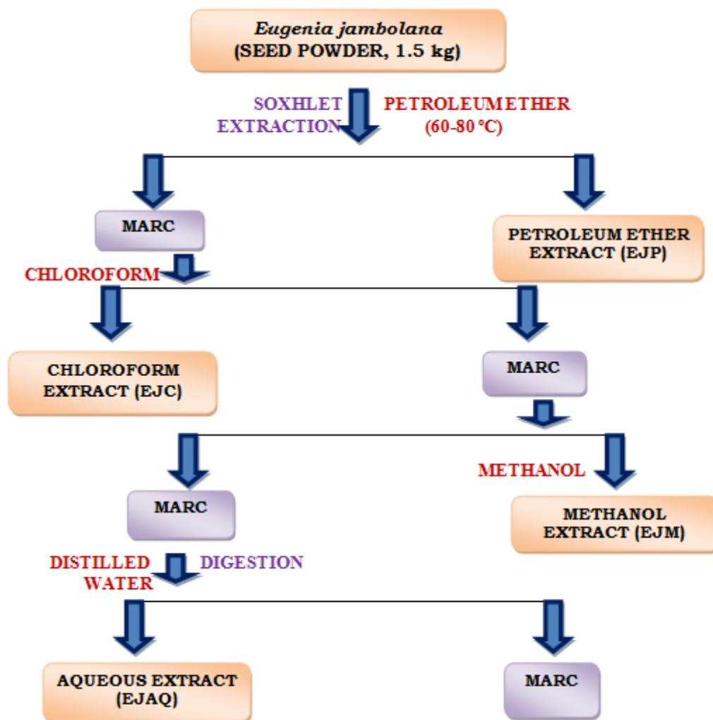
Figure 1: Preparation of different extracts from seeds of *E. Jambolana* by Soxhlet apparatus.
