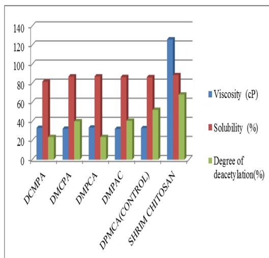
**Fig. 3. Viscosity (cP), Solubility (%) and Degree of deacetylation (%) of crab and commercial shrimp chitosan samples**
