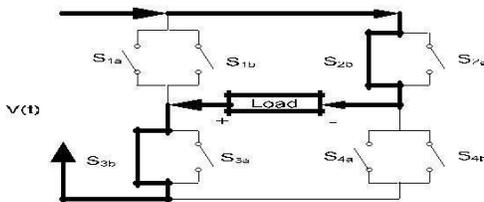
Fig. 10 Providing path for the current to decay in 3<sup>rd</sup> interval
