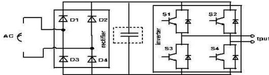
Fig. 1 Conventional rectifier-inverter AC-AC converter
