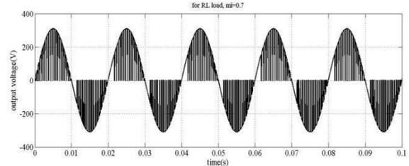
Fig. 20 Output voltage waveform across RL load at 50 Hz, with modulation index,  $m_i=0.7$
