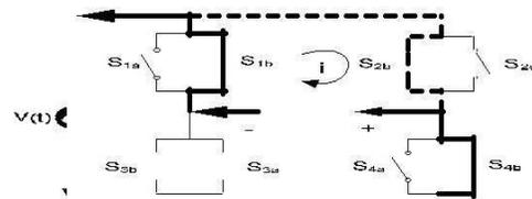
Fig. 13 Inverting and increasing current in 4<sup>th</sup> interval
