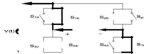
Fig. 5 Providing path for the current to decay in the 1<sup>st</sup> interval
