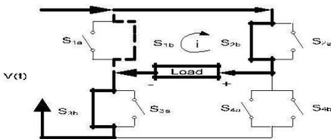
Fig. 9 Inverting and increasing current in 2<sup>nd</sup> interval
