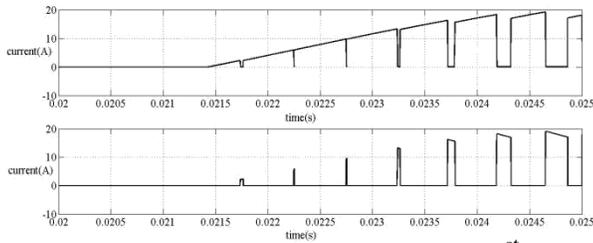
Fig. 7 Current through switches S4a, S2a respectively in 1<sup>st</sup> interval
