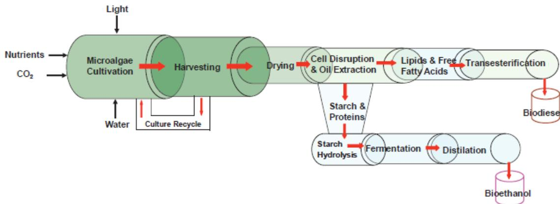
**Figure 3: Biodiesel and Bioethanol production processes from microalgae [2].**
