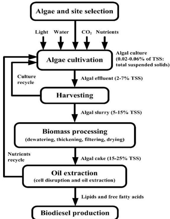
**Figure 4: Microalgal biodiesel value chain stages [9].**
