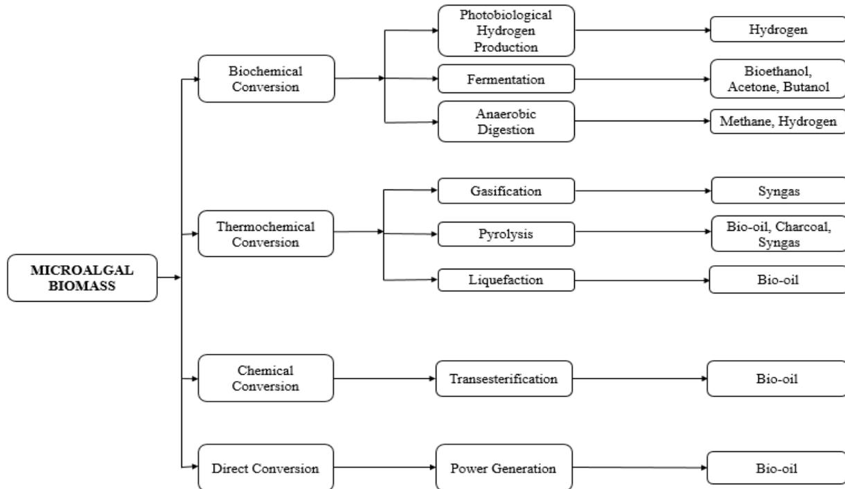
**Figure 2: Biofuel production processes from microalgae biomass [2].**
