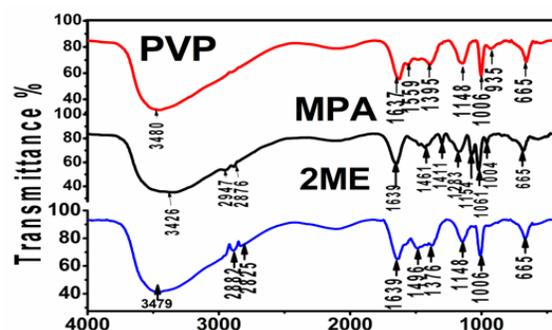
Fig. 4: FTIR spectra of ZnS QDs with PVP, MPA, 2ME as a stabilizing agent.
