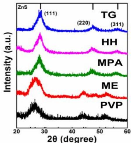
**Fig. 1: XRD pattern of as-synthesized ZnS quantum dots synthesized by using different ligands.**
