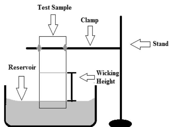
**Figure 1: Wicking Test.**
