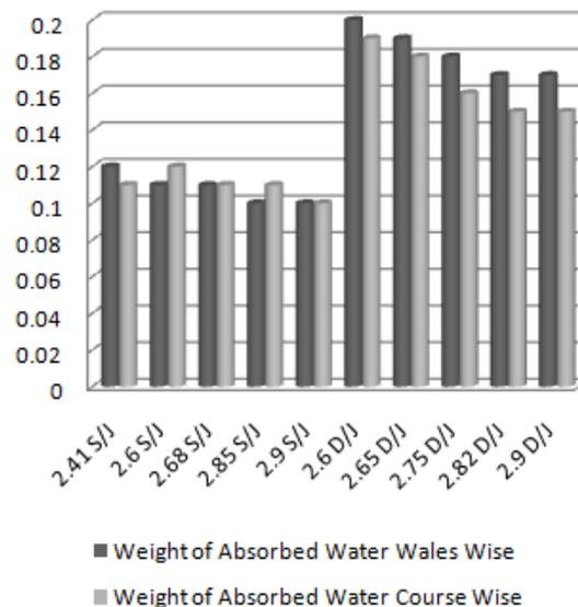
**Figure 4: Absorbed Water by samples Due to Wicking.**
