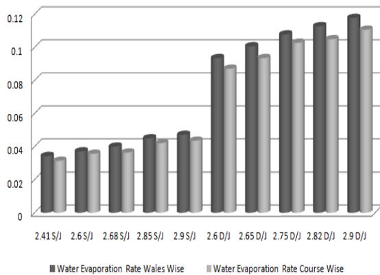
**Figure 5: Drying Rate per Minute.**
