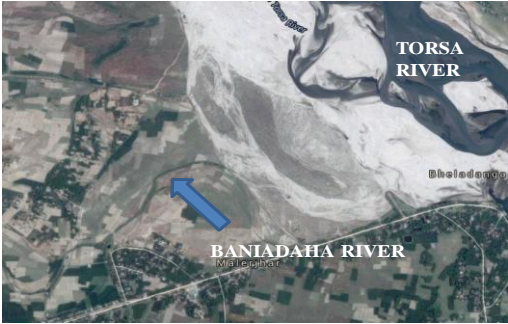
Figure- 5.-Excessive siltation at off-take point of river Baniadaha.
