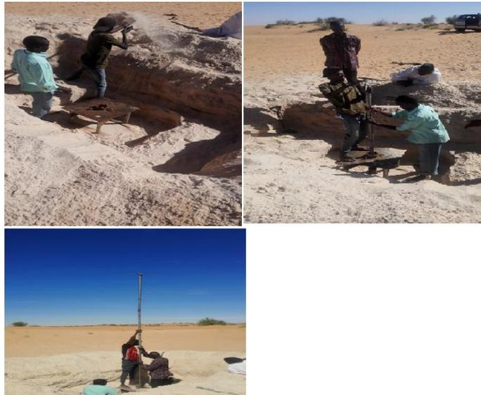
**Plate 3 presenting the Auger drilling during the samples collection**
