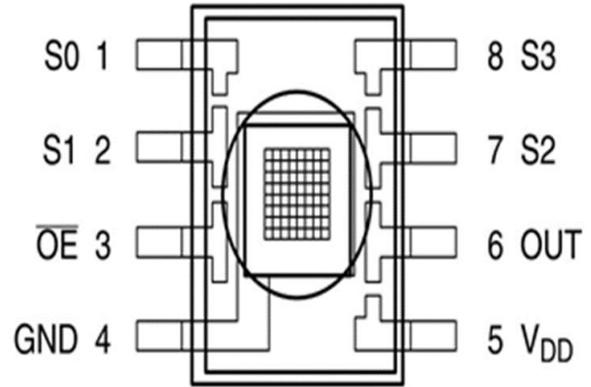
**Figure-3: Internal section of TCS3200**
