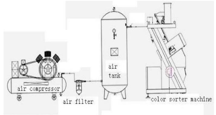
**Figure-5: A reference Pneumatic Color sorting system**
