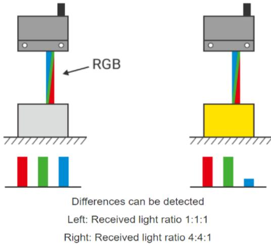
**Figure-1: RGB detection representation**
