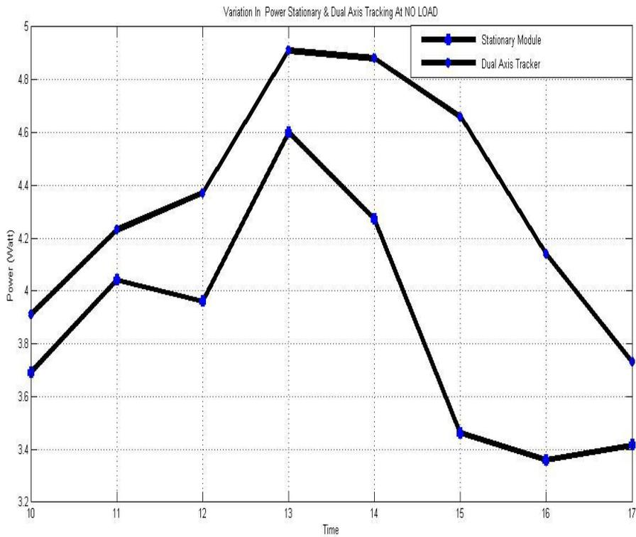
**3.4 Graph between power readings of stationary Solar Panel and Dual Axis solar Power module at load**
