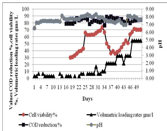
Figure 2: Profile UASB lab scale.
