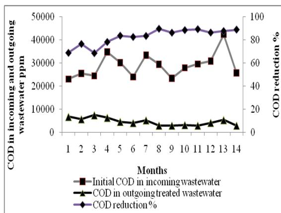
Figure 3: Performance of plant scale UASB reactor.
