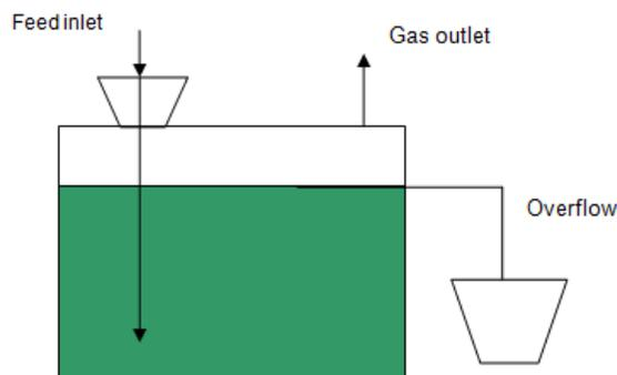
**Figure 1: Schematic diagram of the laboratory scale UASB reactor showing inlet, outlet pipes along with point of venting for gases generated.**
