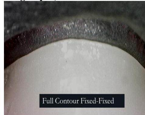
Fig. 4: Vertical margin gap distance of translucent zirconia fixed-fixed bridge (Group I, Subgroup B).
