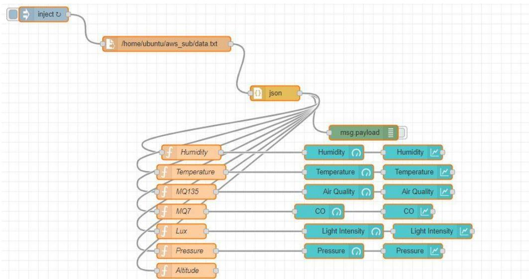
Fig.3. Flow formed using Node-RED
