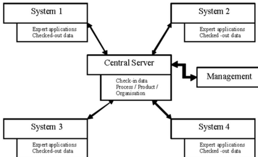
Figure 1 : architecture based on an integrating system.
